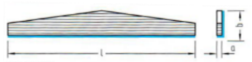
Figure 8: plus grande longueur = l , section totale = a \times b
